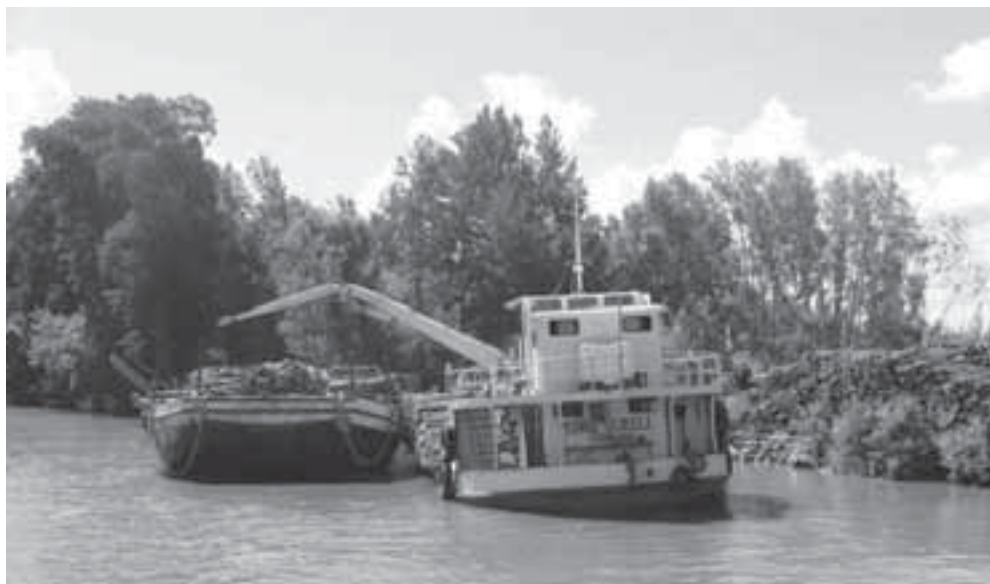
Fig. 5.21. Where plantations are located close to a major river system, barges may be used to transport chips or logs to the mill. Most transport is by barge in the Paraná delta of Argentina; here poplar logs are being loaded on to a barge. Photo courtesy of J. Stanturf.
