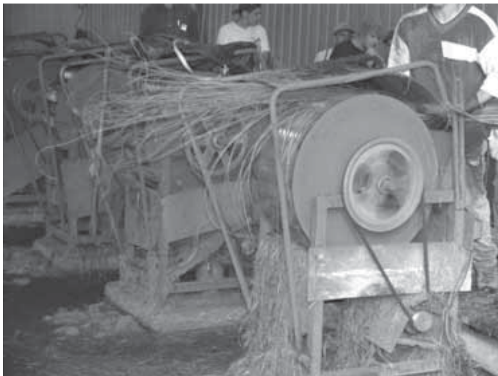
Fig. 5.25. Large-scale processing of basket willow; switches are stripped using specialized machines. Fresh material has been boiled, giving it uniform colour. The next stage is air-drying. Photo courtesy of J. Stanturf.
