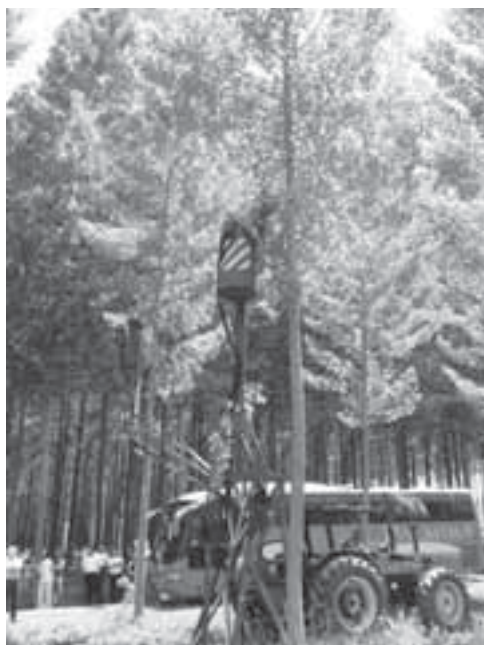
Fig. 5.18. Two workers in tandem, pruning taller trees from hydraulic lifts mounted on an agricultural tractor. Initial pruning was accomplished from the ground using hydraulic shears or small chainsaws on long poles. Photo courtesy of J. Stanturf.
