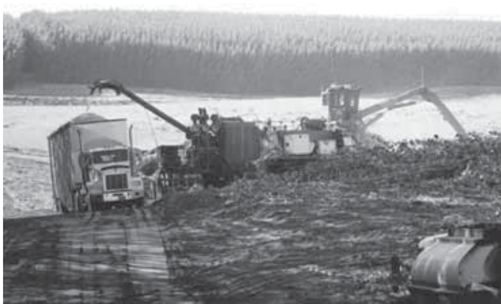
Fig. 5.19. A portable debarking and chipping machine is processing stems at the roadside to minimize skidding to a central chipper. Residual material is consolidated and then shipped for composting or bioenergy production. Photo courtesy of BoiseCascade.
