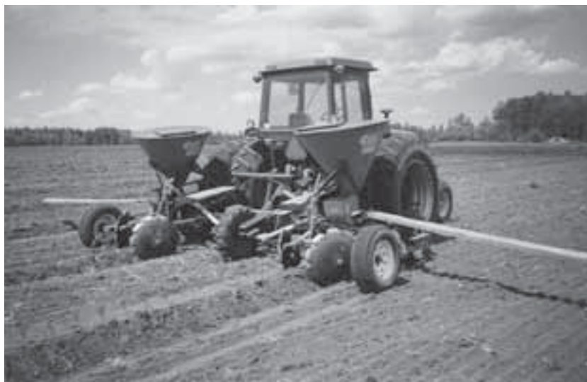
Fig. 5.14. Moulder and fertilizer dispenser pulled by a farm tractor to prepare for planting on former agricultural sites. The fertilizer dispenser is mounted behind a subsoiler shank, which is followed by mounding. Fertilizer is fed by gravity continuously at the bottom of the rip. The disks pull soil into a mound that serves to mark the planting row. Cuttings (45 cm in length) are planted by hand 30 cm deep, right on to the fertilizer. The fertilizer was mono-ammonium phosphate (11-52-0) applied at 220–340 kg ha -1 to supply between 50 and 75 kg P ha -1 . Photo courtesy of Alberta-Pacific Forest Industries Inc.
