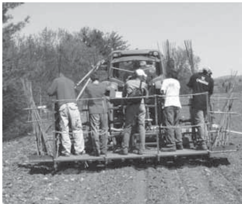
Fig. 5.22. The double-row planting system accommodates use of step planters that can plant two double rows in a single pass. Whips are fed into the machine manually and cut automatically by the planting mechanism into cuttings 18–20 cm long, which are inserted vertically into a slit in the soil made by a coulter; the machine firms the soil around the cuttings. Photo courtesy of N. Thevathasan.
