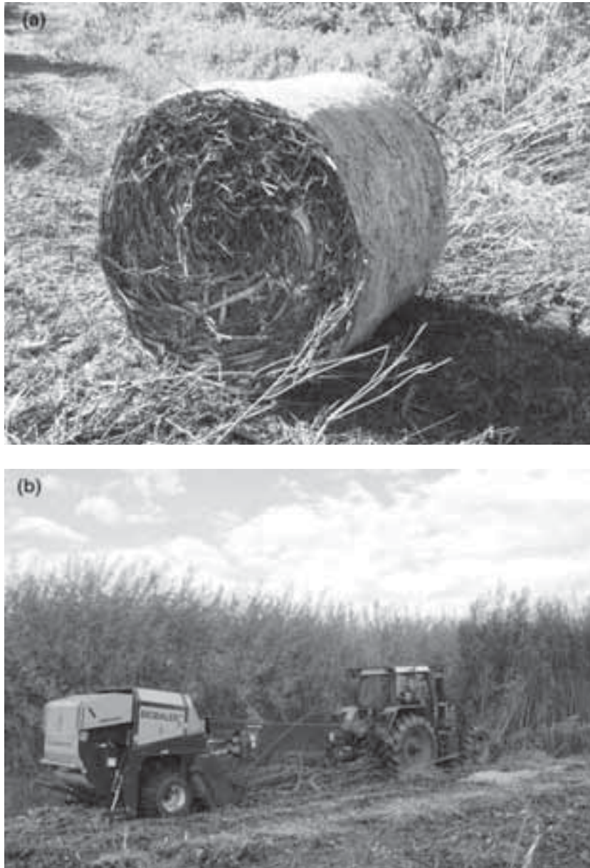
Fig. 5.24. Willow bale produced by the 'Willow Harvester' (a), a prototype bale harvester developed through Université Laval, Agriculture and AgriFood Canada (AAFC) and Natural Resources Canada. These bales are typically 1.20 m in width. The 'Willow Harvester' is a prototype; other balers have been produced commercially and several have been used to bundle biomass from harvest residue in the southern pine region of the USA. 'Biobaler' harvesting 3-year-old coppice willow at Conestota, New York (b). Photos courtesy of C. van Oosten (a) and J. Richardson (b).
