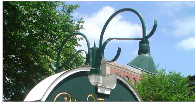
Figure 4.11 A. External Illumination method using gooseneck lamps.
