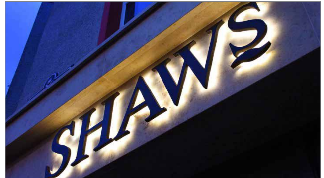
Figure 4.11 E. Example of Silhouette sign lighting. (Image courtesy www.dsigns.com used with permission.)
