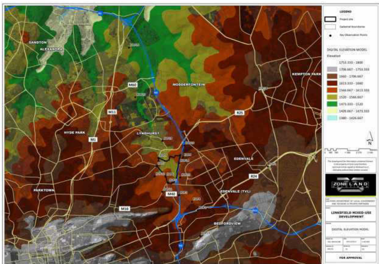
Figure 9: Digital Elevation Model illustrating major ridgelines and dominant view corridors in the sub-region.
