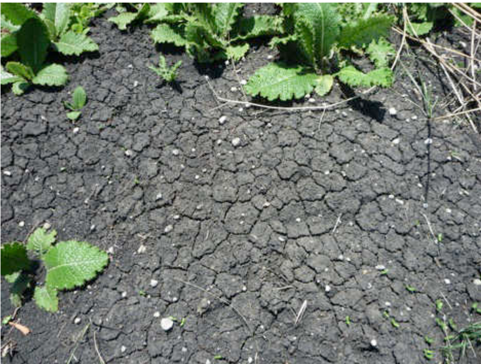
Figure 32 Structured soil in the floodplain of the Jukskei River with swelling properties
