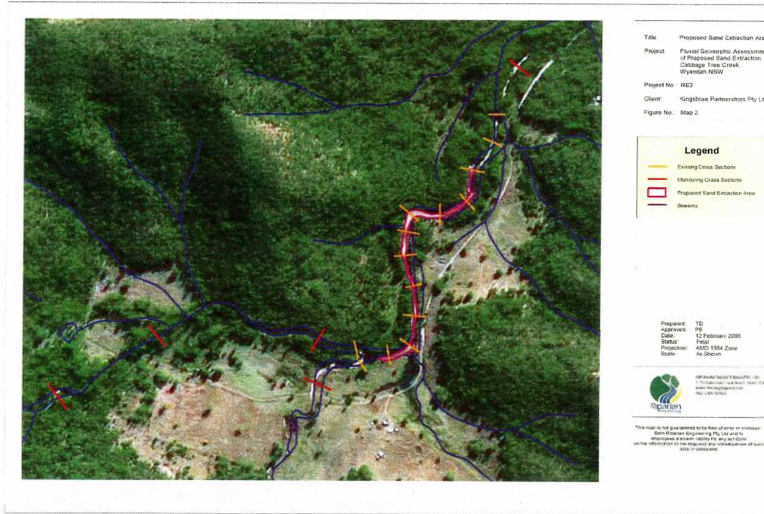
Figure 4. Proposed sand extraction area of Cabbage Tree Creek, existing cross sections, and additional cross sections required for monitoring.
