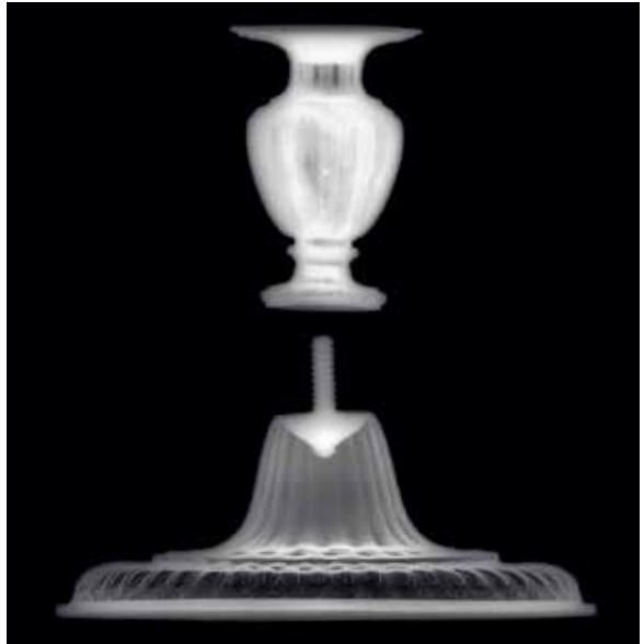
Fig. 11. X-ray radiograph of the thin, hammered foot and thicker, cast stem of the Tiberius figure/Nero dish tazza
