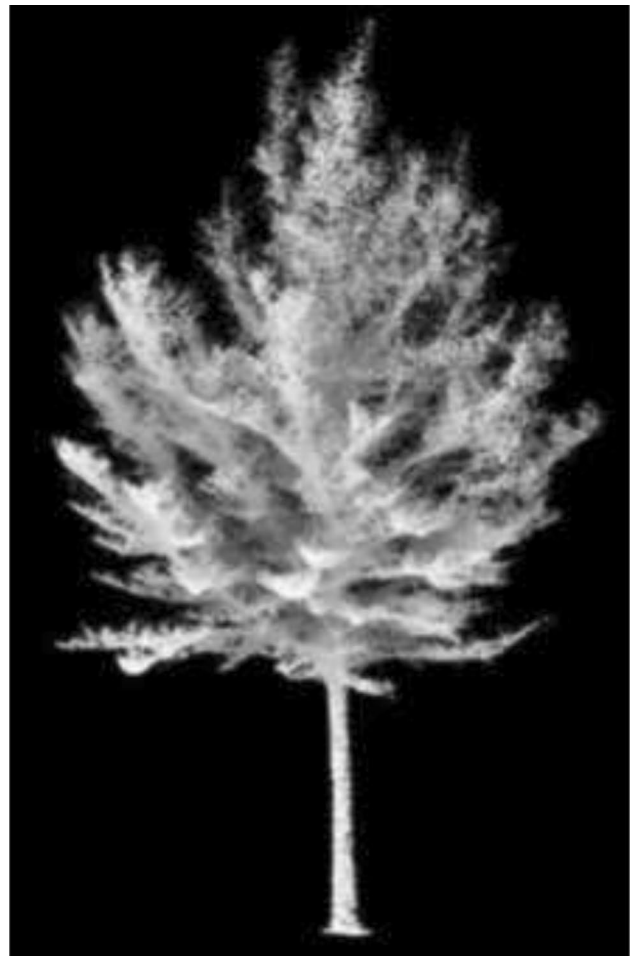
Fig. 3 Exemplary cleaned and filtered 3D point cloud of an Elm tree ( Ulmus ) obtained from mobile laser scanning
