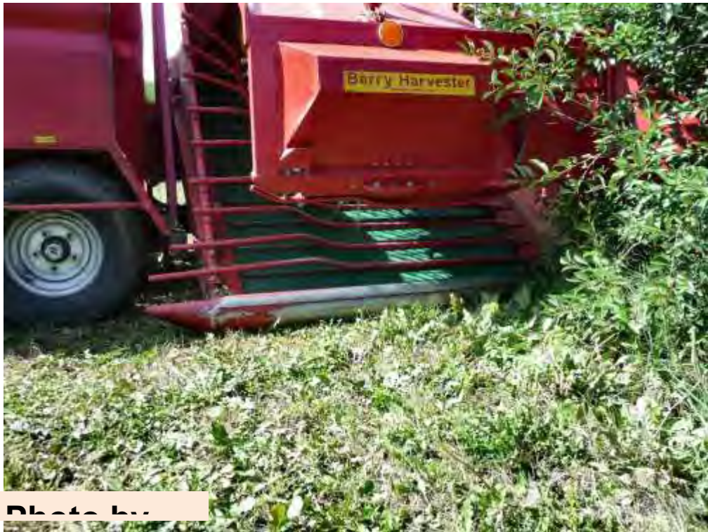
Figure 30. Joanna Harvester with collector lowered to the ground. It is designed to pick fruit just a few inches of the ground
