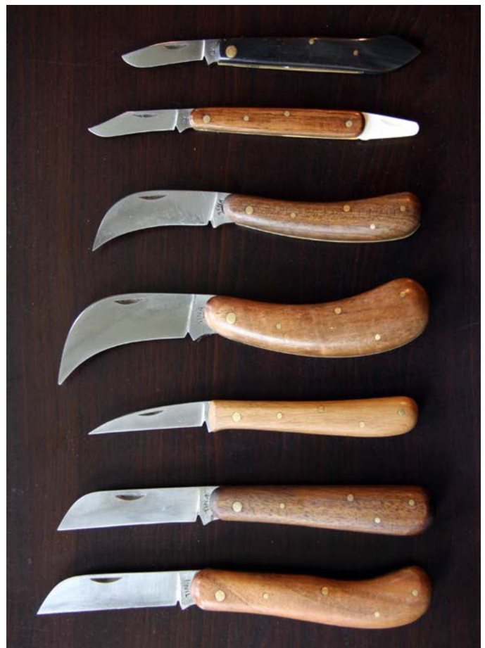
A selection of knives used for budding and grafting, the top two are used for 'T' or chip budding, the curved blades for grafting large calibre rootstocks and scion wood, while the bottom three are suitable for bench and rind grafting
