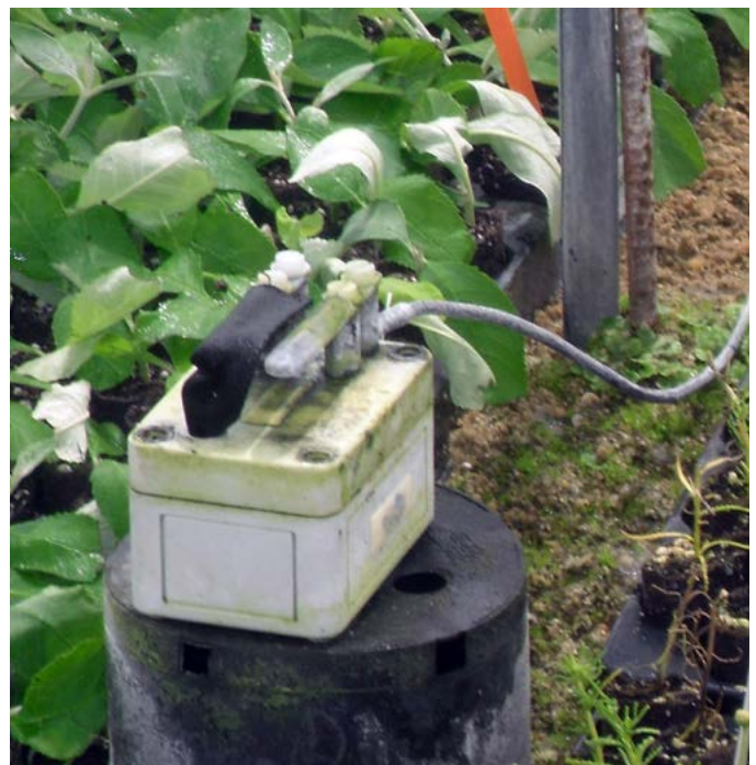
The Evaposensor helps detect and control the evaporative water demand on cuttings in a reliable and reproducible way
