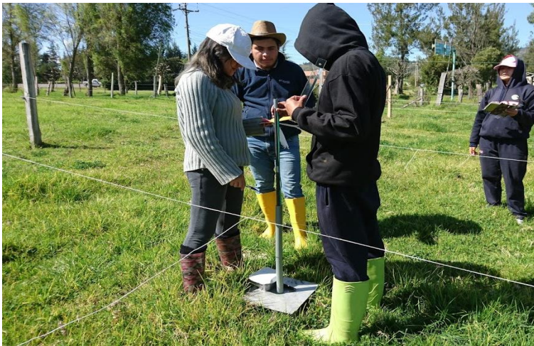
Photo 7. The height of the grass we take in a 30 \times 30 \text{ cm}^2 quadrant with a rising plate meter
