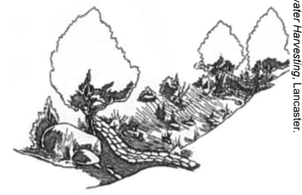
Fig. 10.6. Well-anchored check dams upslope of trees and boulders
