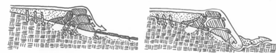
Check Dam with One-rock Dam Apron Vs. Erosion Caused Without
