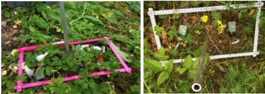
FIGURE 3 A SAMPLING PLOT OF 20X40 CM 2 , DIVIDED INTO TWO HALVES (20X20 CM 2 ), THE CENTER IS MARKED WITH A METAL STAND
