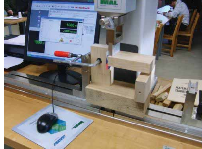
Figure 6: Testing bending strength
