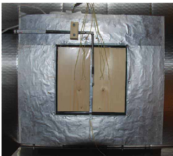
Fig. 2: Housing, samples (covered left, uncovered right) and thermocouples mounted on the ceiling. In center the air speed meter is placed. View from the thermographic camera's position.
