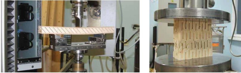
Fig.2. 3- point bending and compression (on the right) test set-up on ZWICK Z100
