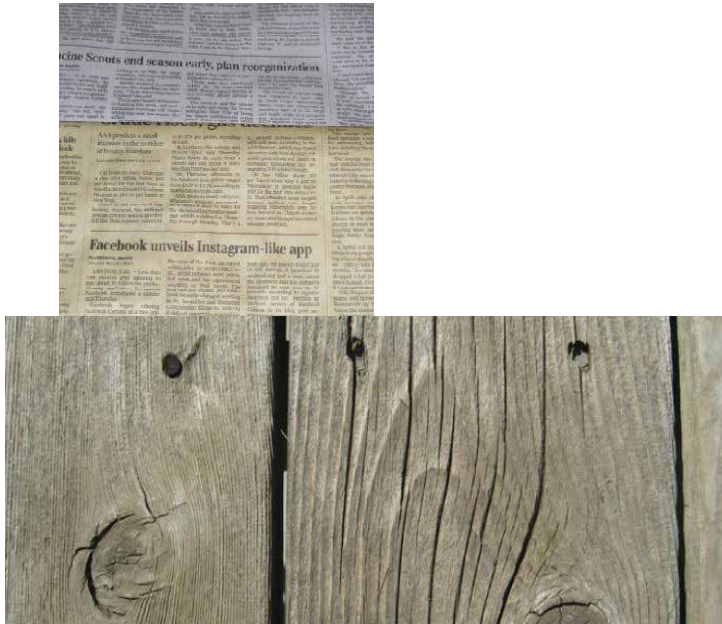
Figure 10 – Change in color of news print and surface checking due to UV energy.
