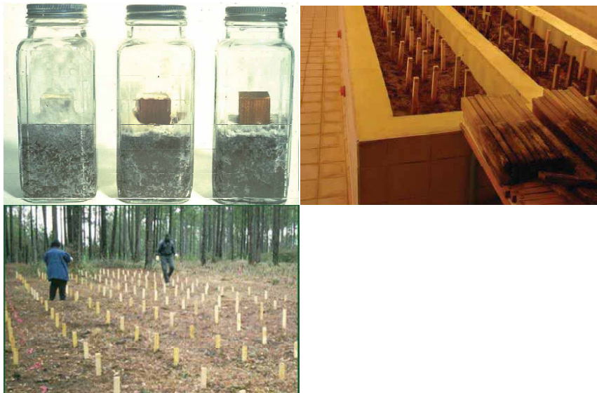
Figure 8 – Tests for wood decay: upper left – ASTM standard soil block test, upper right – fungal cellar test, lower – in-ground stake test.
