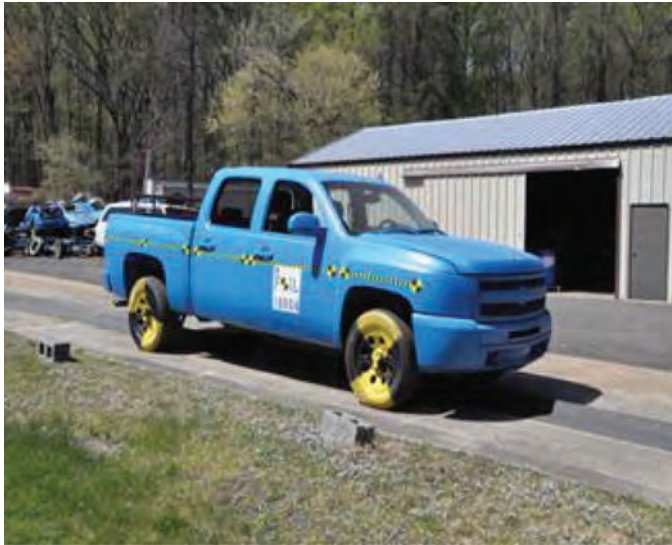
Figure 6.3. Typical MASH 2270P vehicle for crash testing.
