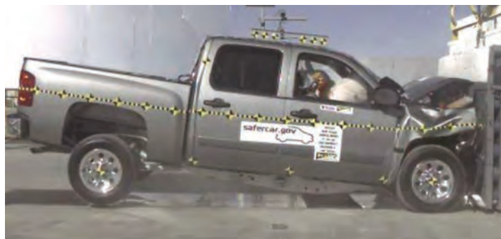
Figure 5.1. Side view of tested vehicle and model after NCAP crash.
