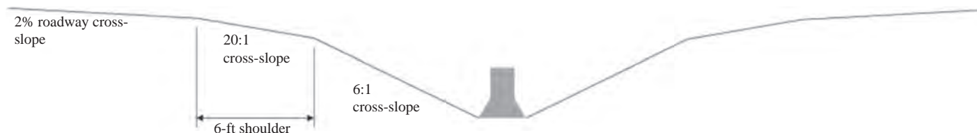
Figure 2.2. Barrier placed in the middle of a 6:1 or shallower sloped median (Sheikh and Bligh 2006).
