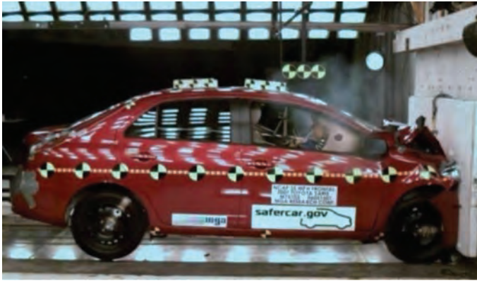
Figure 5.4. Side view of tested vehicle and model after NCAP crash.
