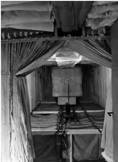
Fig. 1.7 and 1.8: At left, the anechoic chamber with a loudspeaker at the rear (mounted in a panel) and a microphone in front of it. At right, the roof of the acoustics department, with equipment for loudspeaker measurement.
