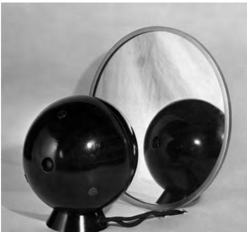
Fig. 1.18 and 1.19: Artificial heads with microphones: at left, a spherical approximation of a real head; at right, a more realistic model.
