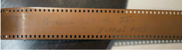
Fig. 2.108: Three-channel 35 mm perforated audiotape dated May 11, 1958, with the final master of the music for the Philips Pavilion; Institute of Sonology archive. Photo by author.
