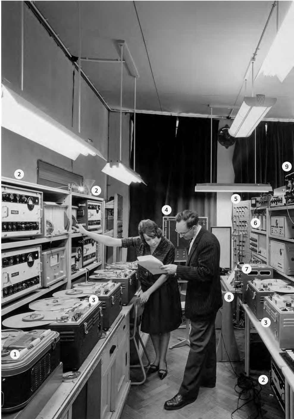
Fig. 3.13: Dick Raaijmakers and Leidi Kiewiet in the Utrecht University electronic music studio, April 1961. In the studio are a Philips EL3516 semi-professional tape recorder (1); amplifiers for Philips EL3509 tape recorders (2); Philips EL3509 tape recorders (3); a patch field (4); a Philips custom-built ring modulator / envelope generator (the same device previously used for the production of "Le poème électronique") (5); a Philips custom-built "characteristics molder" (6); a custom-built tape loop recorder/player (7); an ondes Martenot (8); and a Philips GM2314 impulse generator (9).
