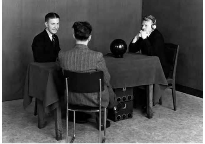
Fig. 1.17: The artificial head was placed on the table. The two amplifiers were set up under the table. The man with the headphones was able to follow the conversation in stereo.
