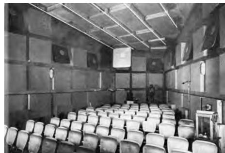
Fig. 1.51 and 1.52: Experimental setup of the Philips reverberation system at the 1954 Gravesano music and electroacoustics conference.
