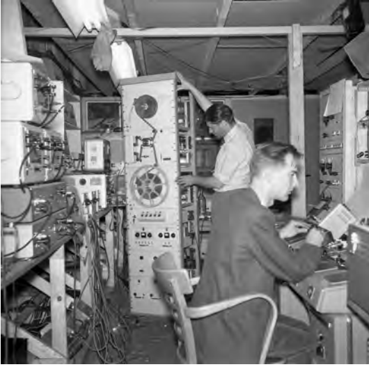
Fig. 2.69: Buczynski operating the three-channel performer and De Bruyn operating a custom-built fader box on top of the EL3800 mixing desk. Photo made with Anton Buczynski's camera.
