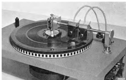
Fig. 1.22: Apparatus designed for stereophonic sound recording on phonograph discs. Each of two chisels was fed signals from one of the microphones on the artificial head. The chisels cut two separate tracks: one in the record's inner zone and one in its outer zone.
