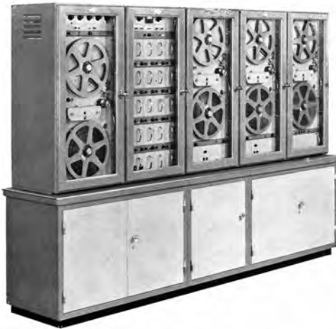
Fig. 2.92: Philips installation for the simultaneous recording of fifteen channels, used, for instance, at air fields to record conversations between air traffic control and planes.
