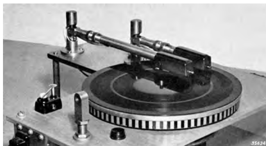
Fig. 1.23: Playback of a stereo recording on a phonograph record with two pickup arms of different lengths to compensate for timing differences between the left and right channels.
