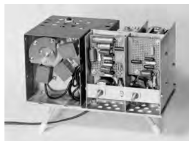
Fig. 1.111 and 1.112: The miniature version of the electronic reverberation system with two playback heads, built as a retirement gift for Vermeulen. The rotating wheel is visible behind the display window on the front panel. An inscription around the display window says "akoestiek - nat.lab 10-10-59."
