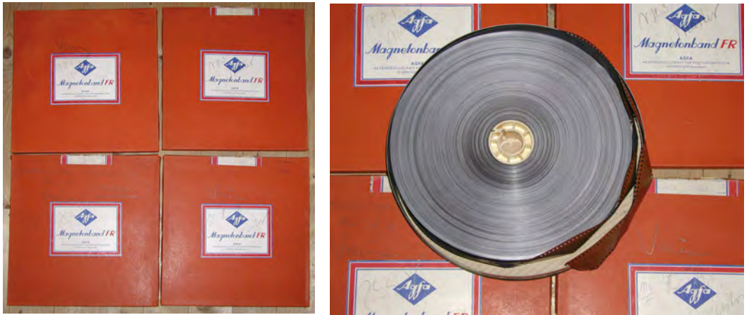
Fig. 2.67 and 2.68: The master tapes of "Le poème électronique" at the Institute of Sonology in The Hague: the three mono tapes and the stereo tape (left), recorded at 76.2 cm/sec, and the three-channel perfo master tape. The German handwriting on the boxes is Buczynski's. Photos by author.
