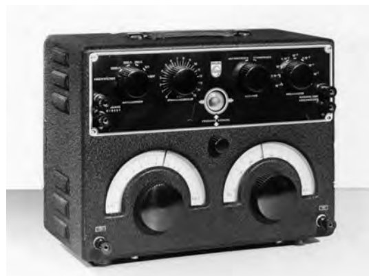
Fig. 1.30: First version of the Philips GM2307 sine wave generator. The large knob on the left was used for the coarse setting of the frequency, the large knob on the right for fine-tuning.
