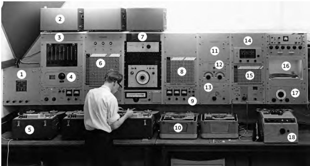
Fig. 3.8: The studio at TH Delft after renovation with echo device (1); amplifiers of Philips 10039 tape recorders with closed lids (2); Peekel TF823 multi-octave filter (3); Siemens Oktavsieb filter (4); Philips 10039 tape recorders (5); patch field 1 (6); Peekel TF273 third-octave filter built around Bruel & Kjaer 1610 (7); patch field 2 (8); tone gate (9); Revox A 36 tape recorders (10); Peekel noise generator (11); Philips GM2307 sine wave generator (12); Peekel sine wave generator (13); radio receiver (14); patch field 3 (15); phonograph (16); Peekel function generator (17); and Revox B 36 tape recorder with variable speed modification (18).
