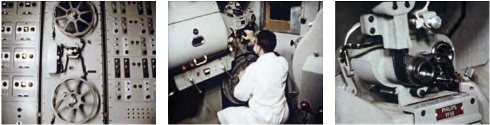
Fig. 2.96, 2.97 and 2.98: The perfo tape machine with the fifteen-channel control tape (left); transporting a film on one of the projectors to the marked point (middle); the film ready to be started by the interlock system.
