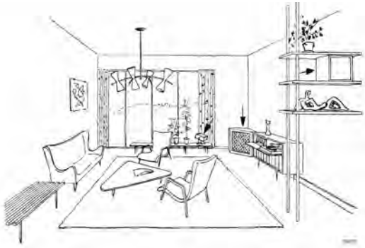
Fig. 1.20: 1950s living room with a loudspeaker for low frequencies in the corner and satellite speakers on the table by the window and on the shelf (see arrows).
