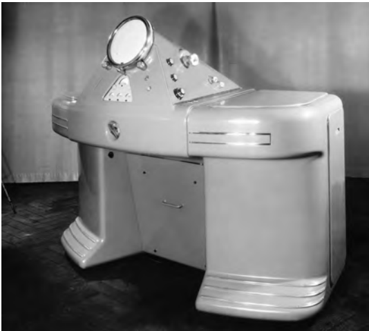
2.70 and 2.71: The Philips electron microscope and an image of a zinc oxide crystal enlarged 32,000 times.
