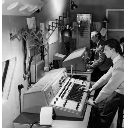
Fig. 2.17 and 2.18: The Grand Auditorium (left) and its control room, with an audio control desk in the foreground, a control desk for incoming radio and television signals, and, at the rear, the artificial reverberation system.
