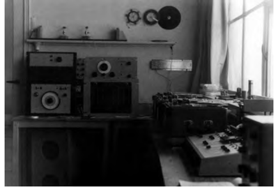
Fig. 3.25: Boerman and Raaijmakers’ studio at Zuilingstraat 25, September 22, 1963. From left: Peekel TF273 third-octave filter built around Bruel & Kjaer 1610, tone gate, Peekel function generator and Peekel TF823 multi-octave filter, all from the former TH Delft studio; spring reverb, three Revox F/G 36 tape recorders, mixing desk built by W. Verschoor of TH Delft, and Philips oscilloscope. Above the filters is the electric monochord; underneath them is a speaker cabinet with two Philips 9710M loudspeakers. Photo by Jaap Spek.
