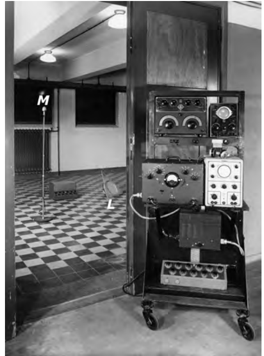
Fig. 1.37, 1.38 and 1.39: Measuring reverberation characteristics (1947). A sound impulse was produced by a loudspeaker (L) and picked up by a microphone (M). The photograph shows the tone generator GM2307 at top left and, under it, the cabinet that generated the envelope shapes of the sound impulses. Next to this cabinet was the oscilloscope that visualized the measurement. The oscillograms show the responses to impulses with durations of (from left) 0.12, 0.07, 0.035 and 0.02 seconds.
