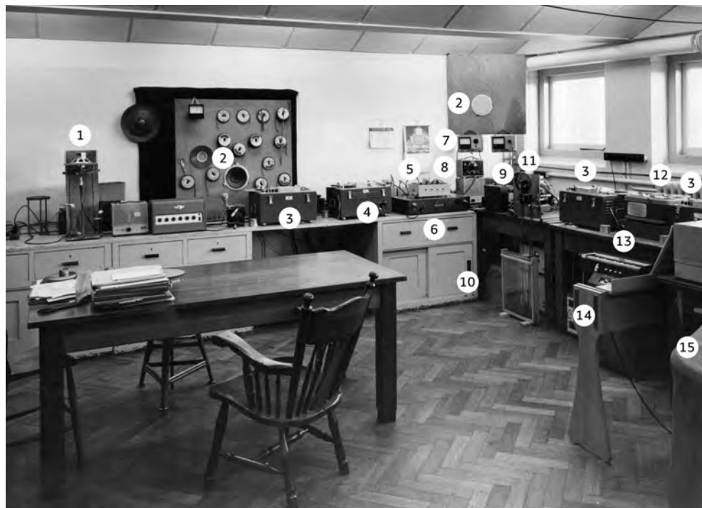
Fig. 1.86: Room 306 in January 1958, containing electronic drum with additional loudspeaker (1); Philips 9710M loudspeakers (2); Philips 10039 tape recorders (3); Philips EL3509 tape recorder (4); fader box (5); octave filter (6); Philips AC millivolt meters (7); Philips GM2315 sine wave generator (8); Philips GM5655 oscilloscope (9); loudspeaker for the ondes Martenot (10); Philips custom-built tape loop recorder/player (11); Philips EL3516 semiprofessional tape recorder (12); ondioline (13); ondes Martenot (14); and grand piano (15).
