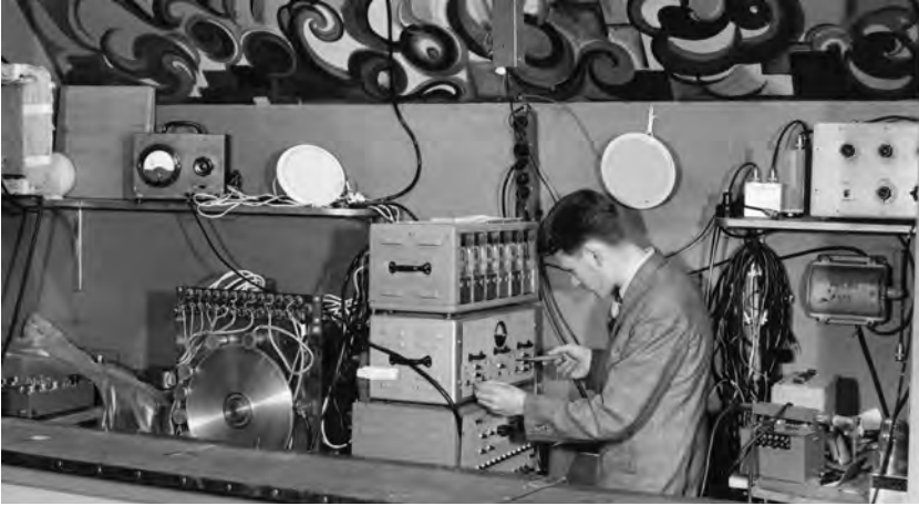
Fig. 1.44: Prototype version of the electronic reverberation system installed in the Gebouw voor Kunsten en Wetenschappen in The Hague. Around the wheel were ten playback heads, of which six could be used simultaneously. The device in the upper right corner was used to create impulse-shaped envelopes. Sound impulses were used in the calibration of the delay times and playback levels of the reverberations.
