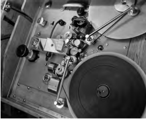
Fig. 1.16: Detailed view of the recording deck with a splicing unit.
