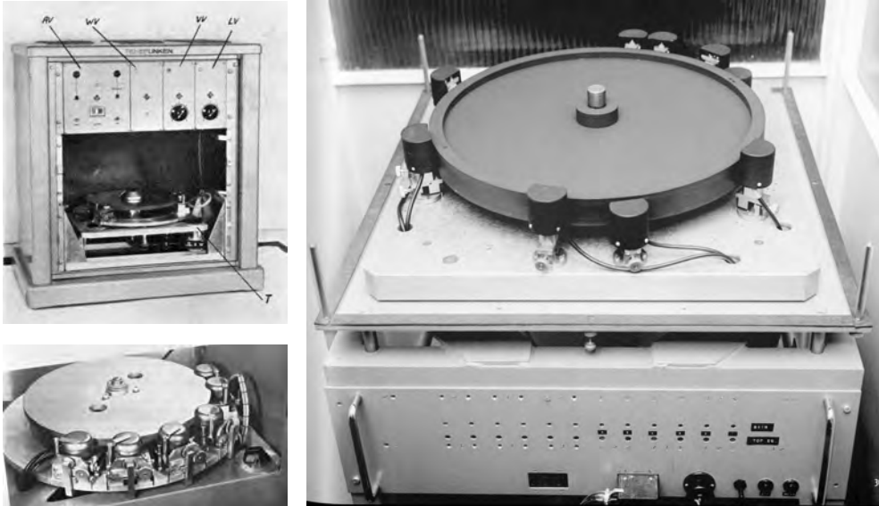
Fig. 1.48, 1.49 and 1.50: Telefunken's time delay unit (upper and lower left) and EMI's delay drum for ambiophonic sound (right).
