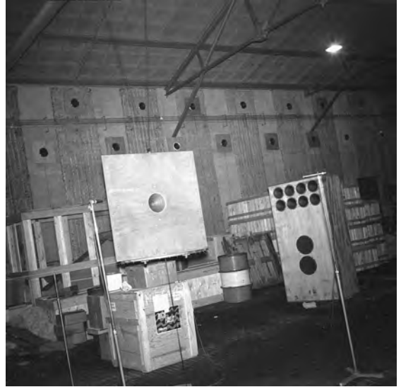
Fig. 2.62 and 2.63: Buczynski in the garage at Strijp III, moving a speaker attached to a rope in front of two microphones (left), and a speaker mounted on a panel with motor-controlled rotation in front of two microphones. Also visible in the right-hand photo is one of the full-range speaker cabinets representing the “antiphonal sources.” Fig. 2.62 made with Anton Buczynski’s camera; fig. 2.63 made by Anton Buczynski.
