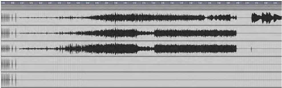
Fig. 2.73: From top to bottom: Track overviews of the three mono tapes and the left and right channels of the stereo tape. At the left are the last clicks for synchronization, followed by "Interlude sonore," then eight seconds of silence, and then the bell sound at the beginning of "Le poème électronique." The stereo tape is silent during "Interlude sonore." Diagram by author.
