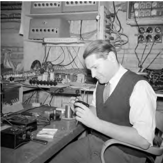
Fig. 2.64 and 2.65: Buczynski working on his electronic panorama control (left) and the connected device after it was completed. Just visible on the left in fig. 2.65 is the stereo tape recorder from Philips’ Phonographic Industries. Fig. 2.64 made with Anton Buczynski’s camera; fig. 2.65 made by Anton Buczynski.
