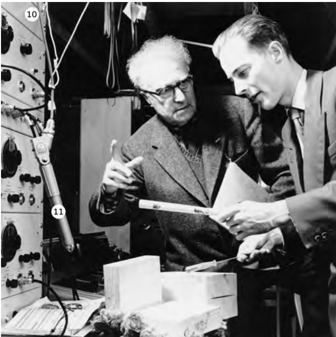
Fig. 2.45: Varèse and De Bruyn in the Strijp III electronic music studio, with Philips custom-built envelope generator/ring modulator (10) and Philips EL6040 microphone (11).
