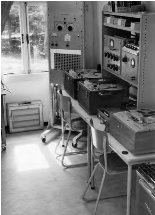
Fig. 3.9: Electronic music studio in the garden house at Gaudeamus in Bilthoven, June 12, 1961. In the corner is a rack from the Delft studio containing, from top, a Peekel noise generator (panel without controls), a Philips GM2307 sine wave generator, an unidentified device, and a patch field. On the table are two Philips 10039 tape recorders and a Telefunken M23 tape recorder.
