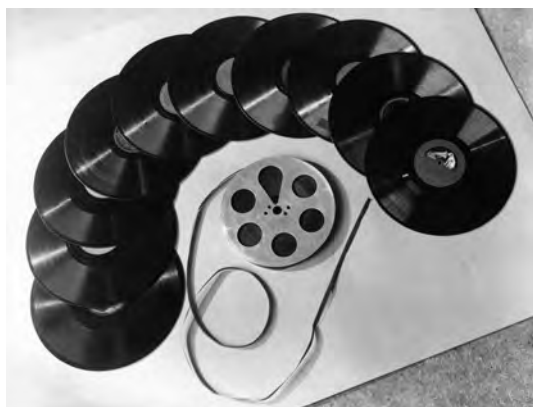
Fig. 1.26: To illustrate the efficiency of recording on cellophane tape, a reel capable of containing an hour of stereophonic music was shown next to the ten 78 rpm phonograph records of 25 cm in diameter needed for the same amount of music in mono.
