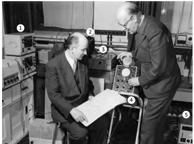
Fig. 1.59: Henk Badings and Roelof Vermeulen in room 306 at Philips Research Laboratories during the production of "Kain en Abel," April 1956. In the picture are two Wandel & Goltermann third-octave bandpass filters with complementary series of bandpass ranges (1); a Philips GM2307 sine wave oscillator (2); a custom-built Philips octave bandpass filter (3); a Philips GM5653 oscilloscope (4); and the amplifier of a Philips 10039 tape recorder (5).
