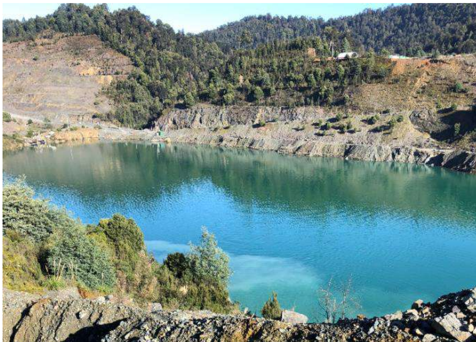
Figure 3-9 – Plume of sediment from underground water pumping looking north to south over South Lens.
