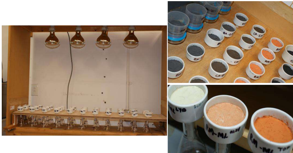
Figure 2. Accelerated kinetic leachate testing on Tasmanian mine waste using mini-Buchner funnels (Moyo et al., 2020).
