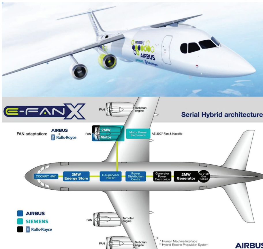
Fig. 6. Experimental aircraft with HBPS Airbus E-Fan X [24]
