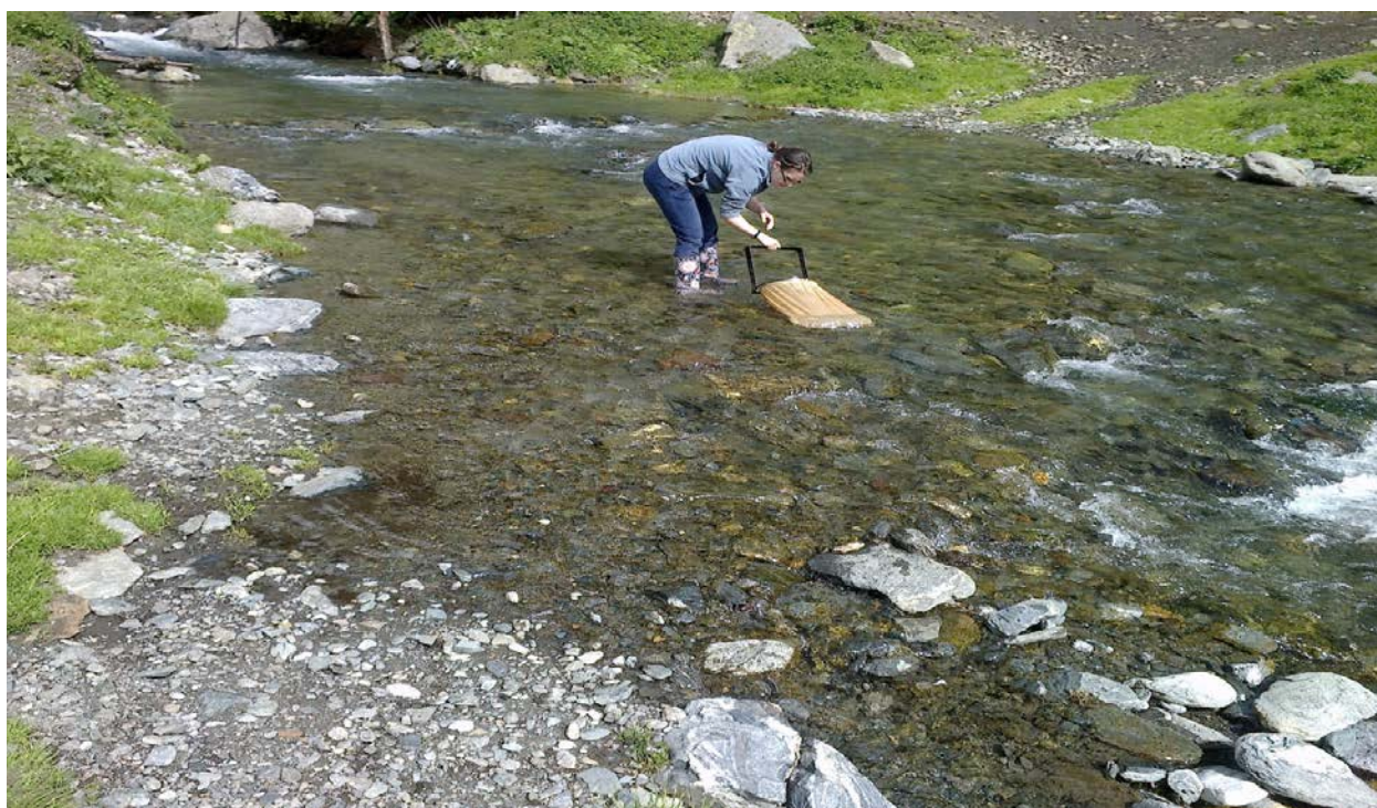
Figure 2: Surber Sampler benthic macroinvertebrates sampling on Capra Stream.
