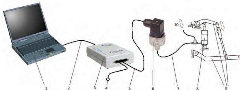
Figure 3. Installation Scheme of Measuring Device PicoLog: 1 – computer with PicoTehnology software; 2 – data cable; 3 – Pico transducer; 4 – DC (12V); 5 – data cabel (4...20 mA); 6 – pressure sensor; 7 – connection tube to hydraulic cylinder; 8 – hydraulic cylinder; 9 – hydraulic hitch-system; 10 – hydraulic oil flow.
