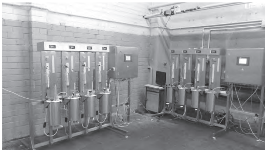
Figure 1. Equipment for biogas yield investigation in the biogas laboratory.
