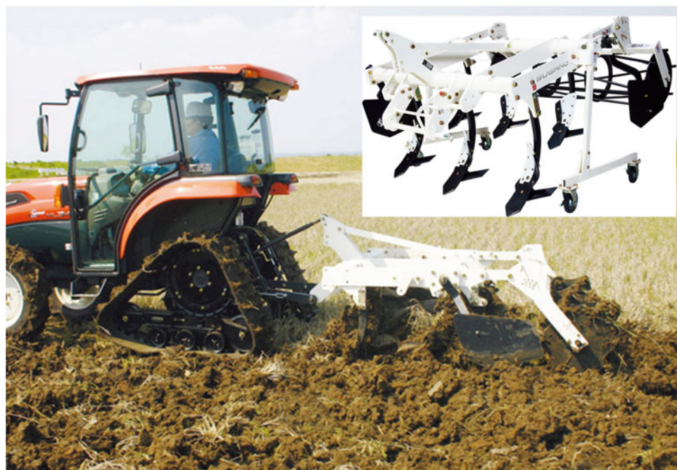
Fig. 10.17 Stubble cultivator (the photo was kindly provided by Sugano farm machinery MFG Co. Ltd. https://www.sugano-net.co.jp/products/stubble/ )
