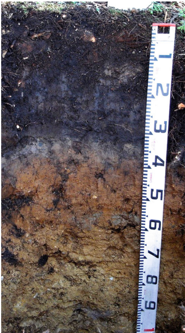
Fig. 4.14 Shimokita soil in Mutsu City, Aomori Prefecture: Podzolized Andosol. Photograph H. Kanno (Tohoku University)
