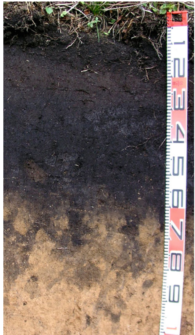
Fig. 4.17 Mukaiyama soil in Oosaki City, Miyagi prefecture: Non-allophanic Andosol. Photograph T. Ito
