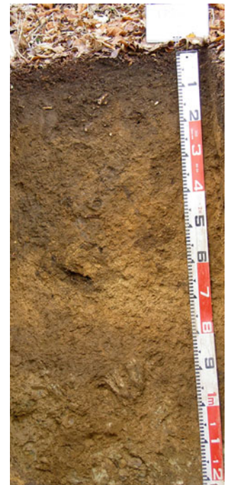
Fig. 4.44 Soil profile of Brown-humic Allophanic Andosol (Typic Hapludand) under deciduous broad-leaf forest in Kyushu Mountains, Kumamoto, Japan Photograph A. Imai
