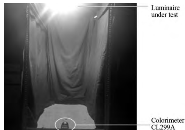
Fig.5. Experimental setup of the colour mixing experiment
