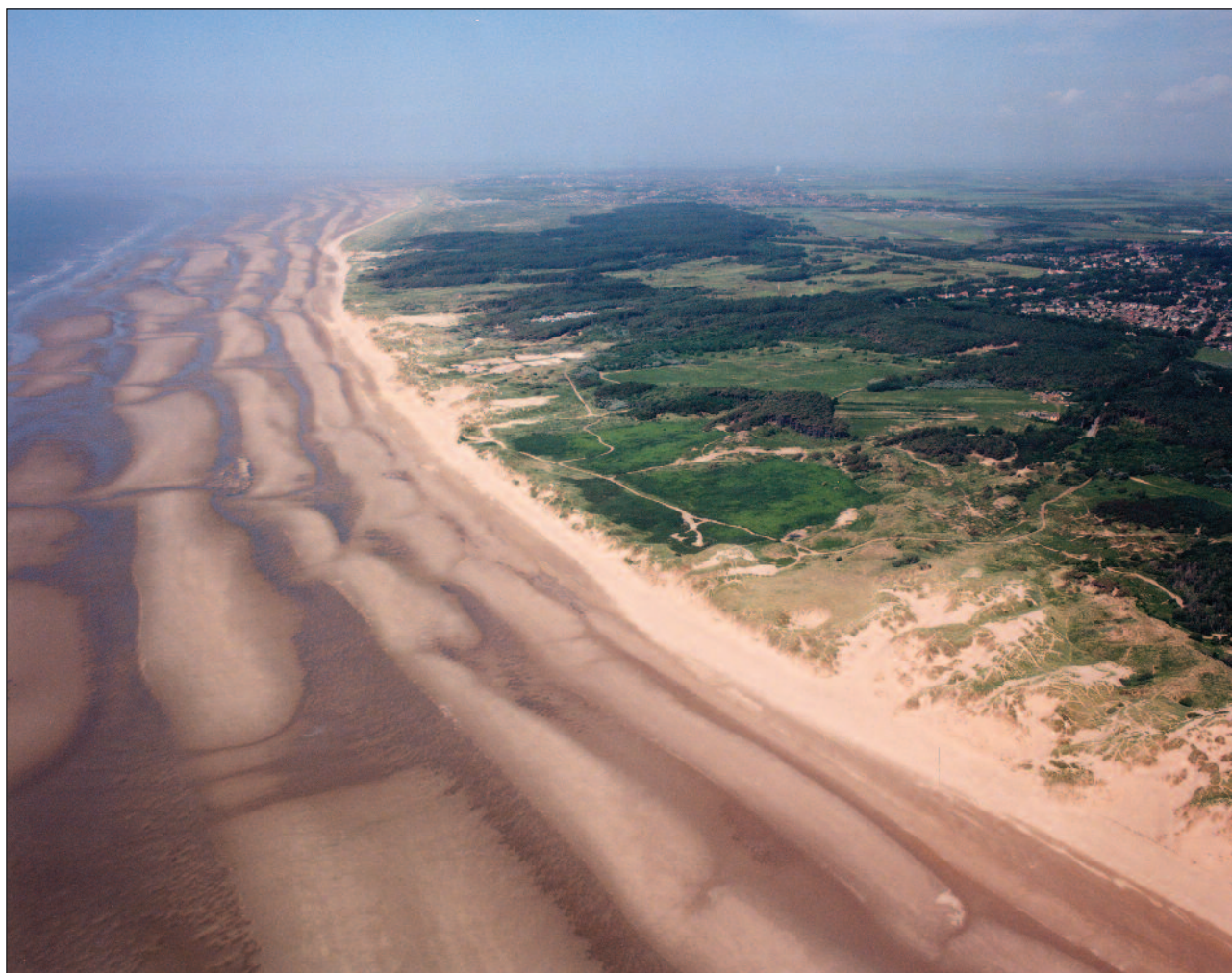
Plate 1. Low-amplitude intertidal ridges on the Sefton foreshore. The figure shows the oblique orientation of ridge crests in relation to the high-tide shoreline, encouraging the net southward and northward drift of sediment alongshore from Formby Point. (Source: Sefton Council).
