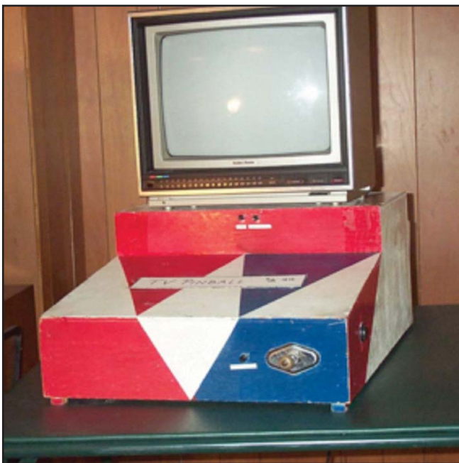
Figure 149- Our TV Pinball Game - Note The Flipper Button (Right) And Ball Launch Plunger (Front)
