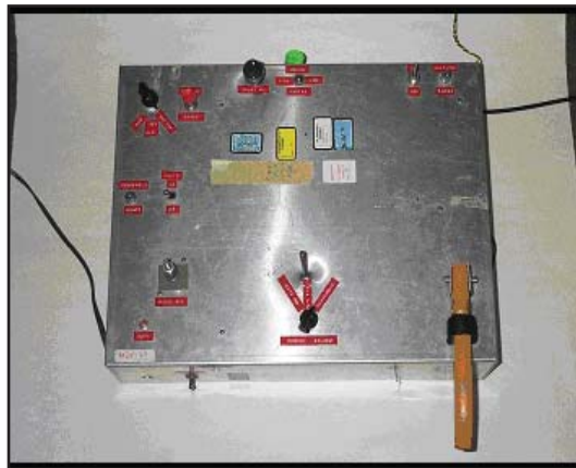
TVG#1 - vacuum tube spot generator
