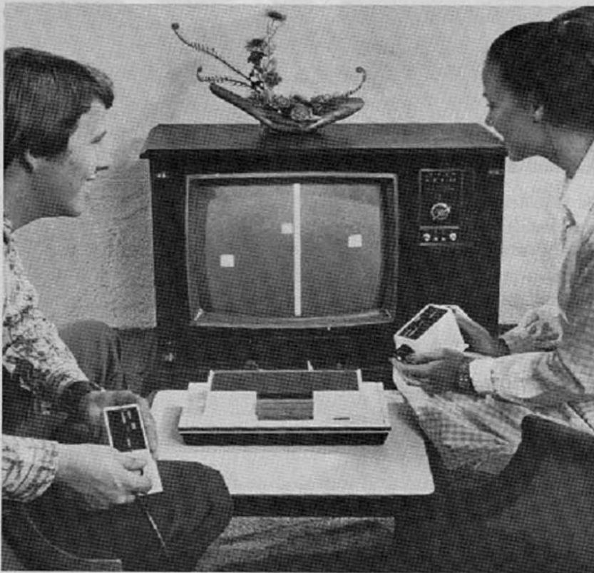
An electronic game simulator that connects to the TV set antenna, by the Magnavox Co., permits TV viewers to play a dozen games of skill or chance. Figures on the screen are manipulated by the contestants.
