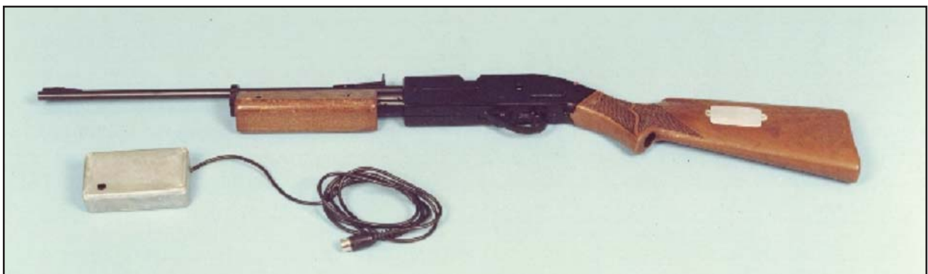
Figure 151 - The Precision Rifle Along With The Small IR Data Receiver That Plugged Into The Apple IIe Computer
