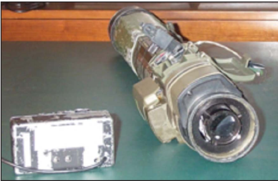
Figure 152 - The M72A2 Light Antitank Weapon (LAW) Modified For Emulation Training
