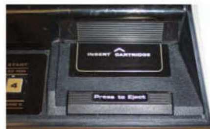
» The cartridge port was capable of taking large cartridges that were a similar size to the 8-track tape cartridges that were popular at the time.
