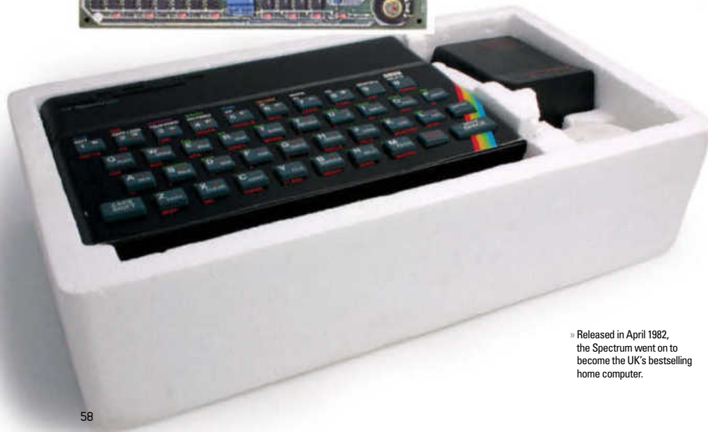
» The Spectrum was a fairly simple machine, with no dedicated graphics hardware and limited expansion options. (photo: Bill Bertram)
