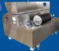
Industrial FCPC® 15 L machine for production (ATEX cGMP standards)
