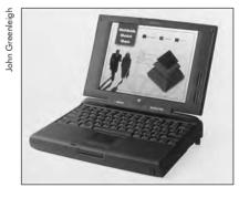
The PowerBook 5300 series marked the debut of PowerPC-based portables, but flaming batteries and cracked cases required several recalls to fix.
