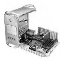
The Power Mac G4 with mirrored doors was very easy to expand thanks to its foldout side.
