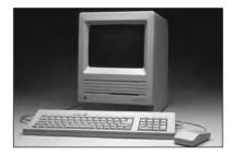
The Mac SE was the first model with an optional internal hard drive and PDS (processor direct slot); hence the name, which stands for "system expansion."
