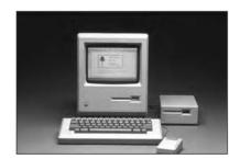
The Mac 512K (shown here with an optional external 3.5-inch disk drive) was nicknamed "Fat Mac" because it came standard with four times the memory of the original.
