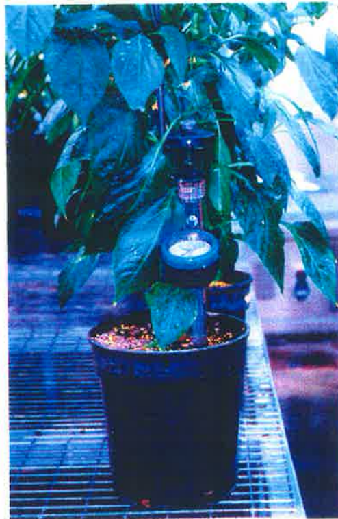
Figure 5.1 Tensiometer installation to a depth of 11 cm into the soil for measurement of the soil moisture potential.
