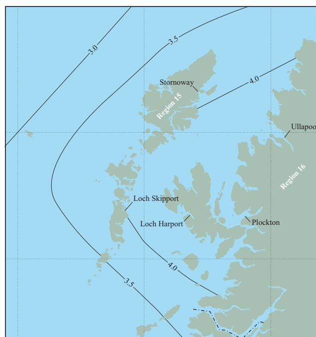
Map 2.3.5 Tidal range (m) at mean spring tides. Source: Lee & Ramster (1981). © Crown copyright.
