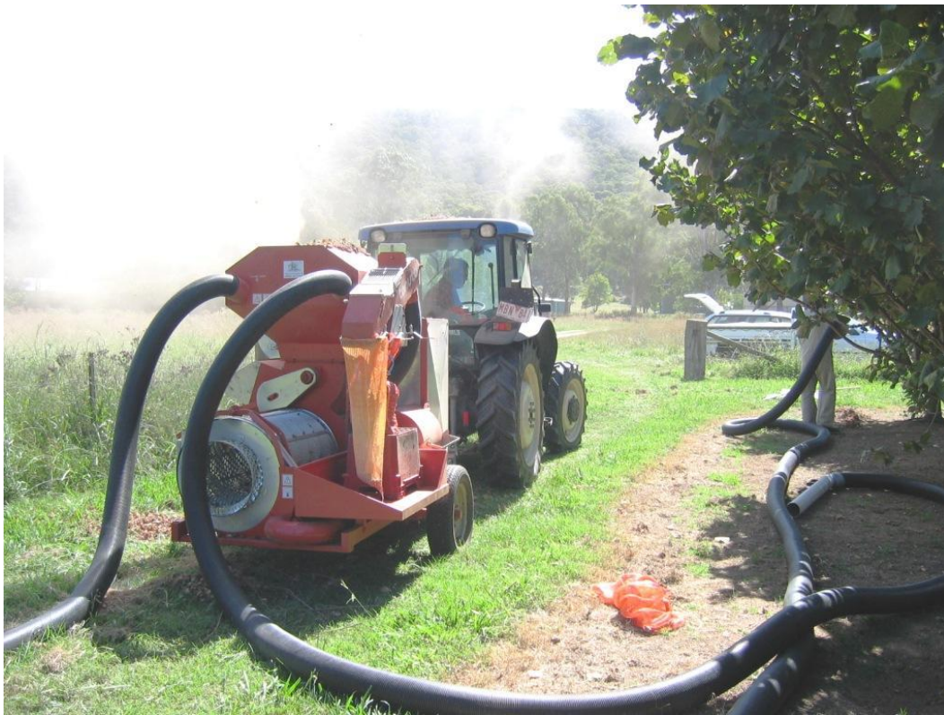
Plate 7.1 Tonutti vacuum harvester used for collecting nuts at Myrtleford in March 2005; All trees were harvested separately to obtain nut yields.
