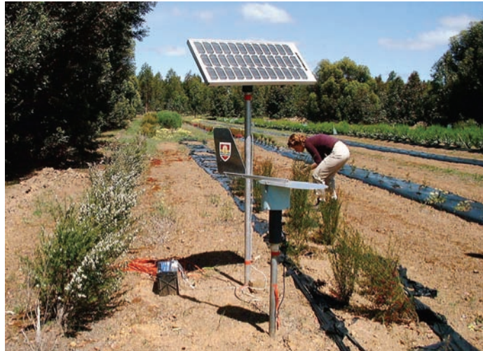
Split-type volumetric spore trap set adjacent to trial plants located at Mt Barker (WA).
