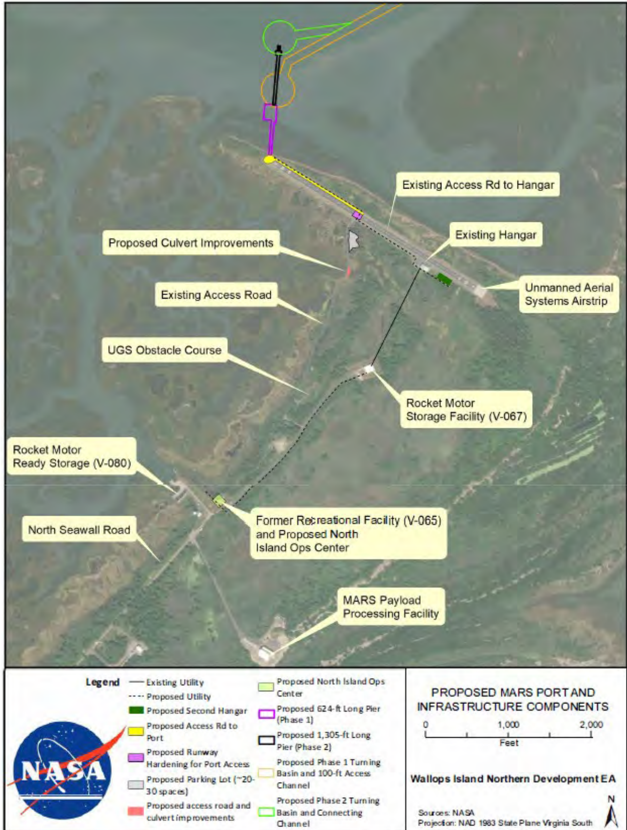
Figure 2. Proposed MARS Port and Infrastructure Components
