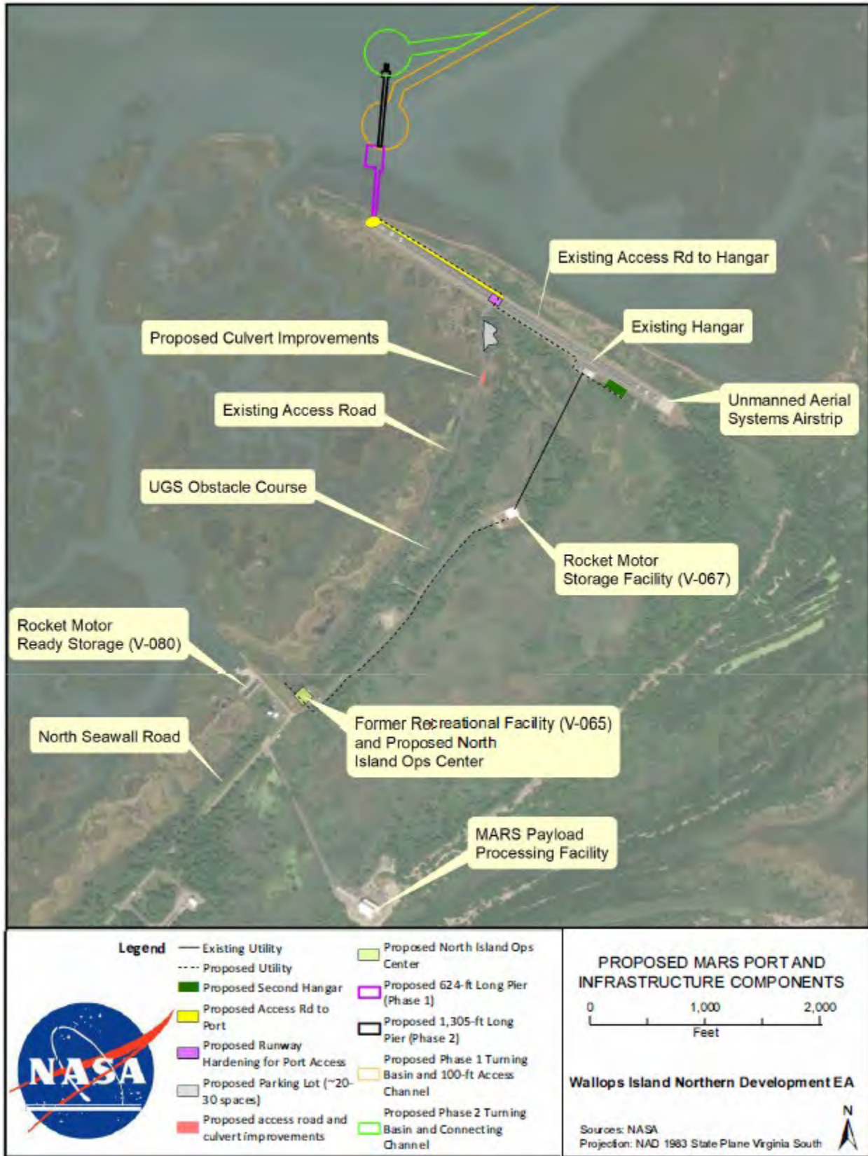
Figure 2. Proposed MARS Port and Infrastructure Components
