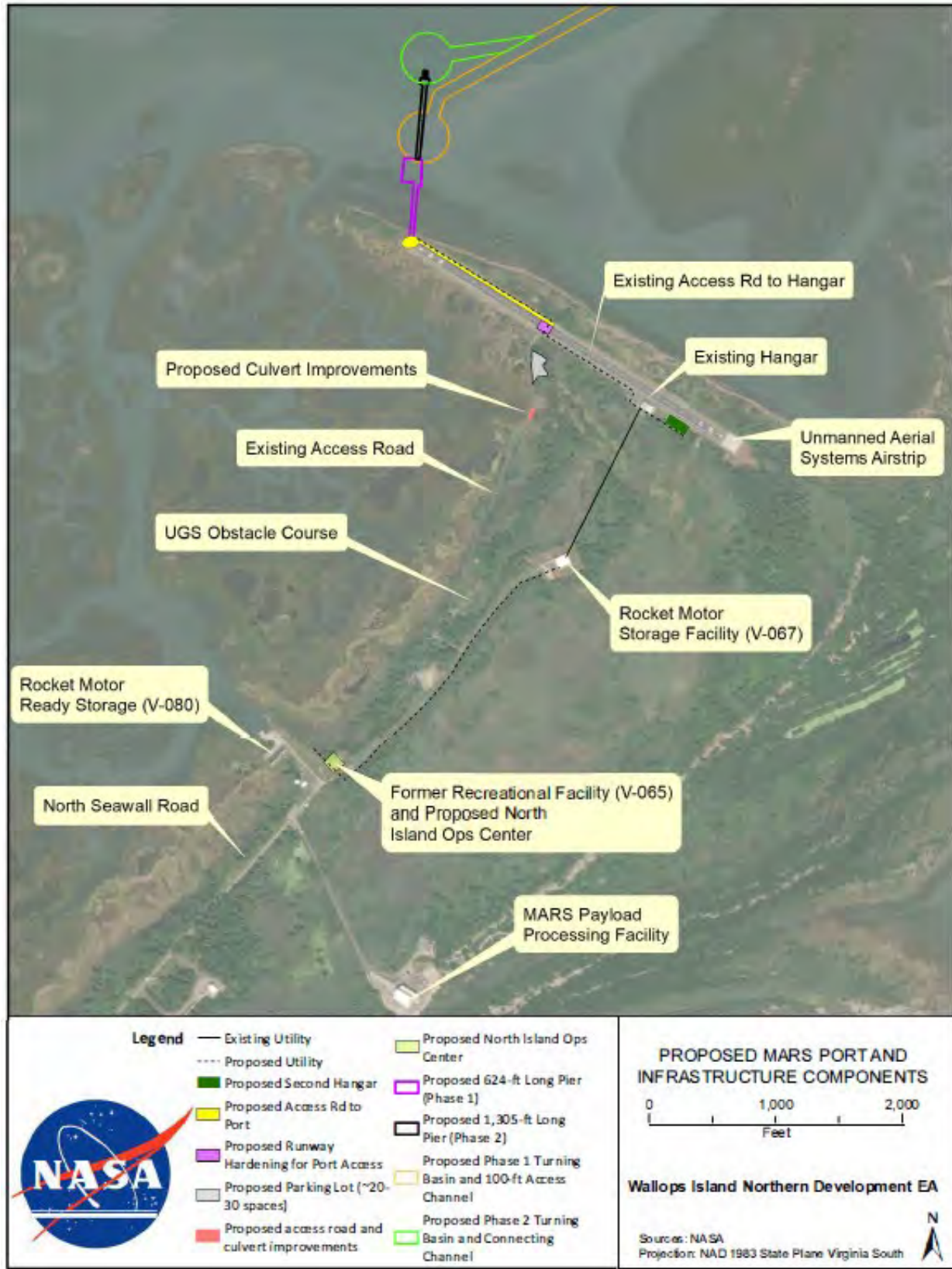
Figure 2: Proposed MARS Port and Infrastructure Components
