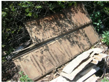
Figure 59: Metal sheeting showing pressed metal roof tile pattern.
