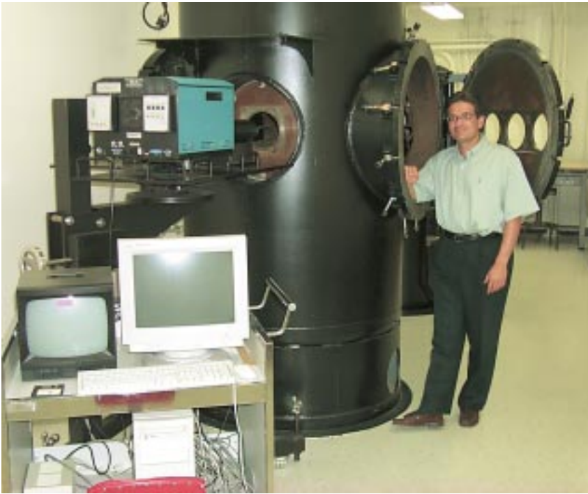
Above: Rosakis and a high-vacuum target chamber being modified for use with the digital camera (the blue-sided box at upper left). Built for plasma-jet studies in 1963 for the late Professor of Aeronautics Lester Lees, and later used by von Kármán Professor of Aeronautics, Emeritus, Anatol Roshko (MS '47, PhD '52), the chamber wouldn't look out of place on a battleship—just the ticket for confining hypervelocity shrapnel.
