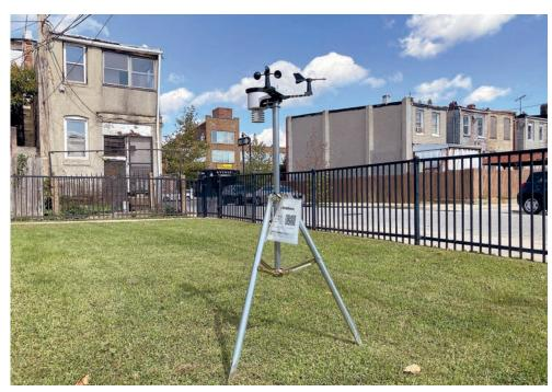
A weather station in eastern Baltimore monitors temperature, precipitation, humidity and sunlight. Instruments to measure soil moisture are being installed by Morgan State University. (Timothy B. Wheeler)
