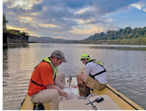
*Hydrologic technicians for the Pennsylvania Water Science Center collect water samples from the Monongahela River near Braddock to be tested as part of a statewide survey for PFAS chemicals in surface water. (Lowell Abbadini)*
