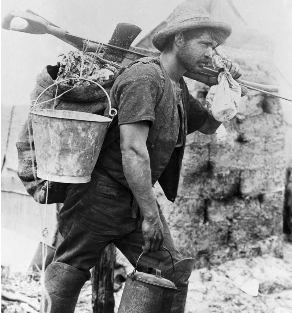
Figure 6-14. Northland New Zealand gum digger fitted out with a spear for prodding the soil for kauri resin, a bucket for sluicing, a billy for midday brew, and a knapsack, or pikau, for carrying the day's haul. The small flour bag in the digger's hand was kept handy for storing small pieces of resin he found while digging for larger chunks. With permission of the Alexander Turnbull Library, National Library of New Zealand, Te Puna Mātauranga o Aotearoa (Northwood Collection, negative G 9781 1/1).
