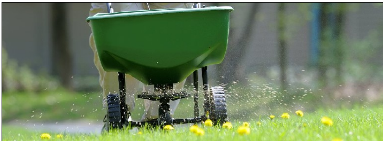
Image of someone using a broadcast spreader to apply a granular product to a lawn.
