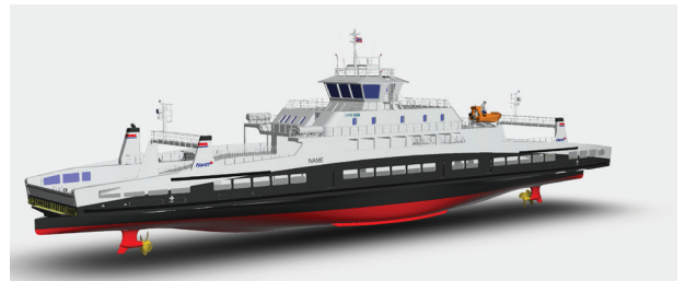
Illustration: HAV Design. Double-ended ferry with Brunvoll Azimuth Propulsion
