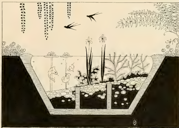
A cross-section of the concrete-lined pool shows the sloping arrangement of the soil and the partitions to hold it in place
