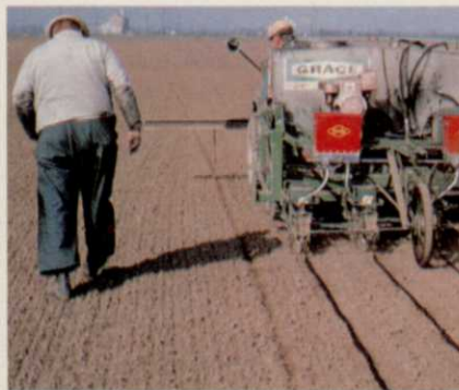
2. Charcoal banding is a process where the seed and liquid fertilizer are layed in rows and sprayed with a band of charcoal covering the seed. The charcoal protects the seed from Karmex or Atrazine applied to kill weeds.
