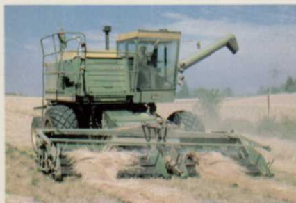
9. Combines mechanically separate the seed from the straw by a series of rubbers incorporated in the thrashing machine.
