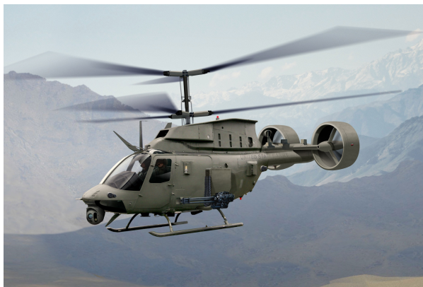
Figure 2: AVX is currently refining its proposal for the U.S. Army Future Vertical Lift (FVL) aircraft, developing a Coaxial Compound Helicopter concept shown in figure. Photo courtesy of http://www.avxaircraft.com .
