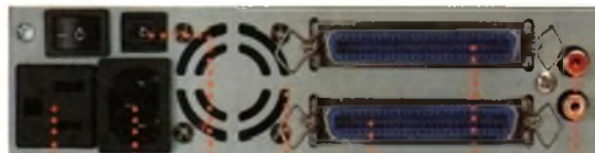
110V 240V SCSI ID SWITCH COOLING FAN SCSI CONNECTORS AUDIO IN/OUT
