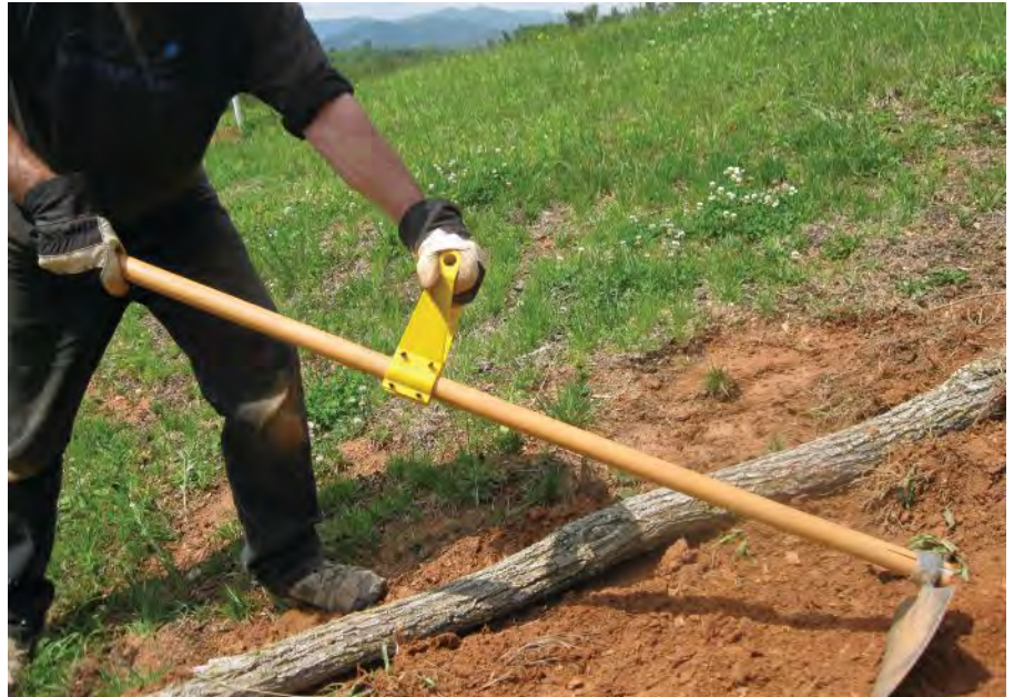
Attached to the handle of a hoe, Stout's Back Saver Grip reduces strain by increasing leverage.
