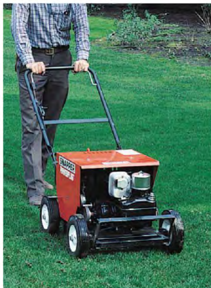
Soil aeration counteracts the negative effects of compaction in a lawn. A power aerator, left, accomplishes the job by extracting small soil plugs, above.
