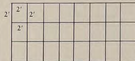
PERIMETER CLOSURE—192 FEET
