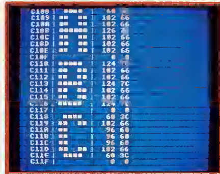
Top: Part of the BBC micro's bit map. Below: Enlarged letters displayed from the micro's ROM.
