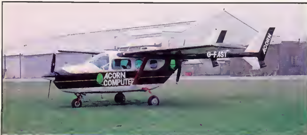
NO, Acorn isn't going into competition with Virgin has two engines, one behind the cockpit, the other in the front. The Cessna can carry six people, just the equivalent to the Presidential plane. It's a Cessna thing for transporting high-flying millionaires 337 'push me, pull you', so nick-named because it
