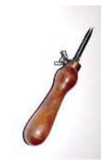
The handle of a stitching awl made of service tree wood from Moravia (2, 2012).
