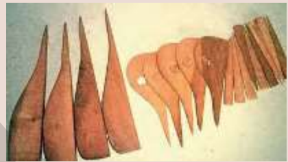
Various forms of "piquettes" made of service tree wood, designed for cutting paper rolls; central France (3, 2009).
