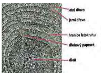
A transverse section of the trunk of a service tree, adapted (Schoch et al., 2013).
