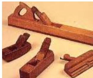
Historical jack planes wholly or partly (sliding surface, peg) made of service tree wood (5, 2007).
