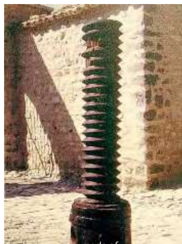
Wine press screw made of service tree wood from the 18 th century, Salagon Museum, France (4, 2009).
