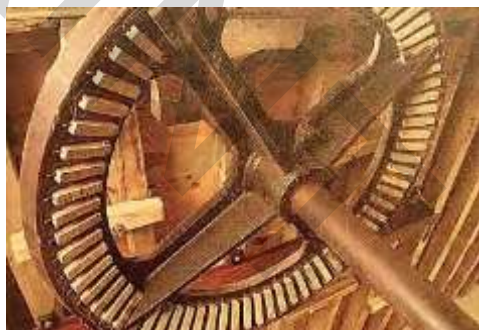
Wheel tothing of the restored mills in la Sarthe, France, is still made of service tree wood (4, 2009).
