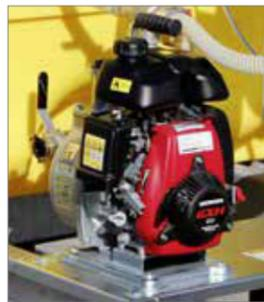
Motorpumpe HONDA 130l/min
