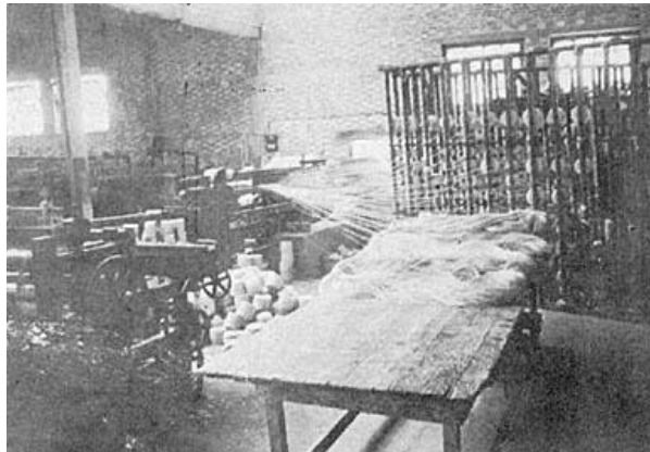
The Caroa is spun into a tough cord for sacks, in the Jose Vasconcellos factory in Pernambuco, Brazil
