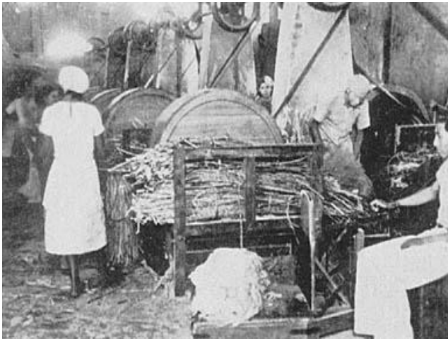
Collected leaves of Caroa are fed through rollers which crush them, then these fibres are decorticated.
