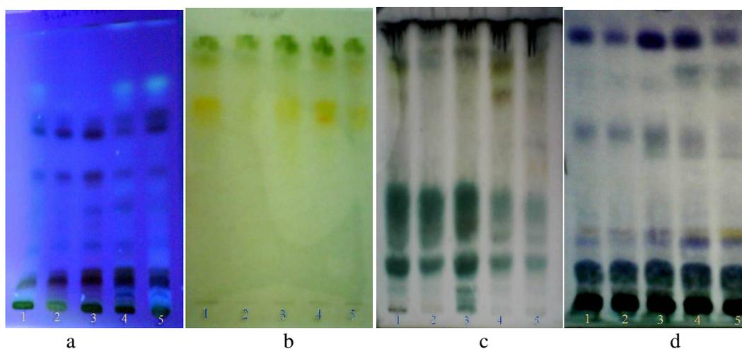
**Figure 5.** The chromatograms for polyacetylenes- UV (a), tannins (b), saponins (c) and volatile oils (d).
