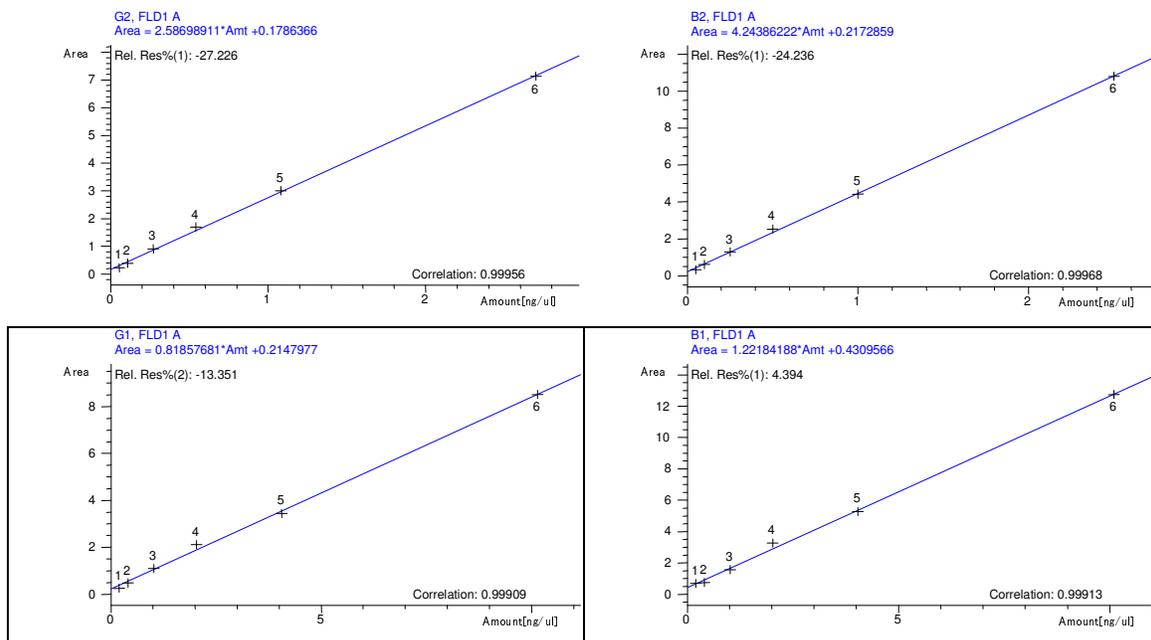
**Fig. 2.** Calibration curves of aflatoxins
