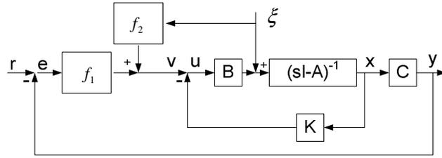
**Fig. 2.** Structure of the nonlinear control system
