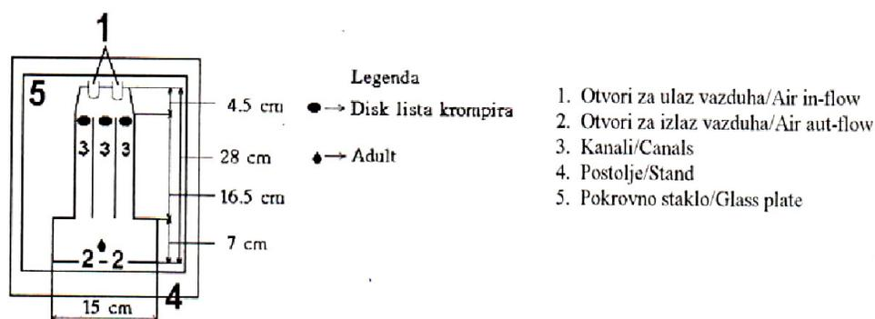
In order to function, the olfactometer uses the air pump and rubber-coated tubes (9 mm in diameter) for the inlet air to the manifold, the air flow regulator, the rotameter and the glass air hub with activated charcoal (which served to neutralize the odoriferous substances in the air). The air velocity through the rotameter was ca. 2000 l/h (i.e. 0,55 l/s), while in the olfactometer itself the air speed was ca. 75 ml/s.
