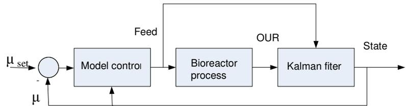
**Figure 1** Block diagram of the control algorithm
