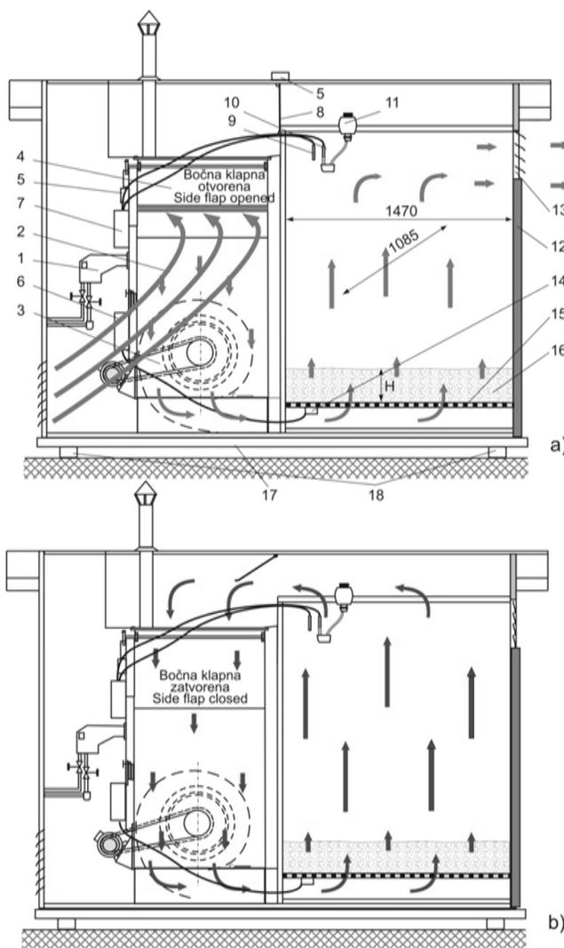
**Figure 1** Experimental dryer, a) open mode, b) circulating mode
