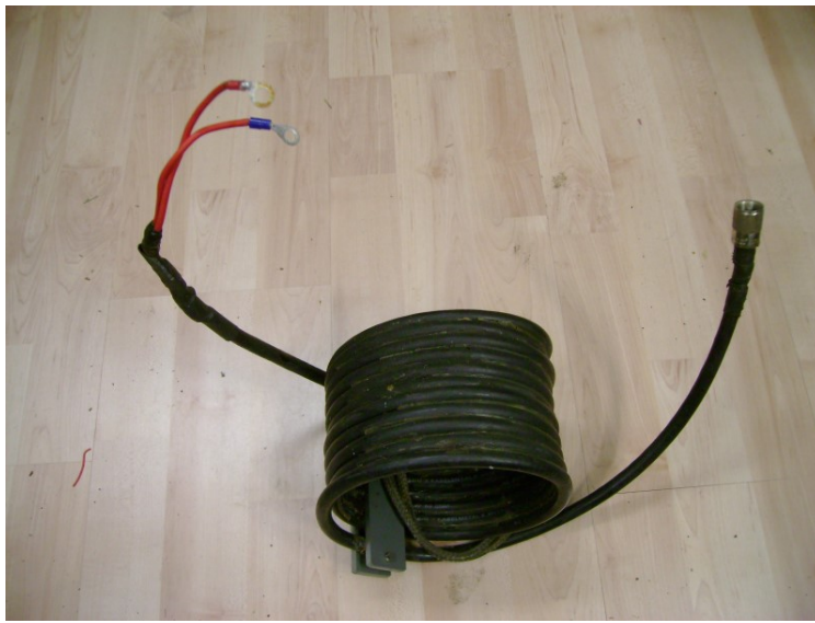
Figure 6.9 Ten turns of RG213 as a current balun
