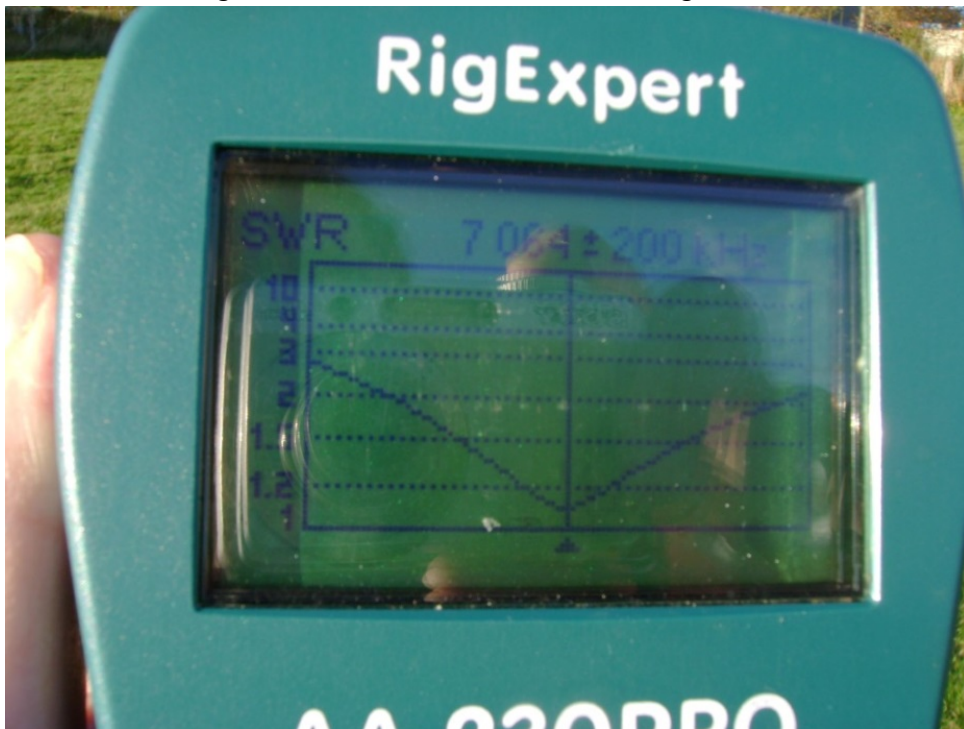
Figure 6.4 SWR of a 40m 4-square element on 7064 \pm 200 KHz
