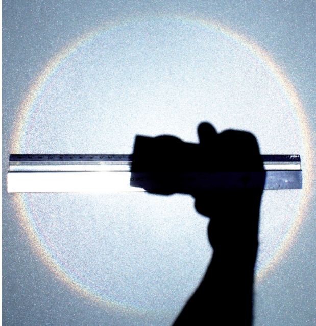
Figure 10. An aura above a layer of \mu Beads is shown through polarizing filters. The spectral halo, best described as a three-dimensional rainbow of colors, was the result of upward projections of light by refraction through millions of \mu Beads spread in a 2 – 3 mm layer over a flat 1 m 2 level concrete area. A 30 cm ruler spans the diameter of the circle of light and the black silhouette is of the author's camera and forearm. The hemisphere is brightest toward its center; moreover, all points of the 1 m 2 covered with \mu Beads were approximately 20% higher in PAR intensity than adjacent surfaces.
